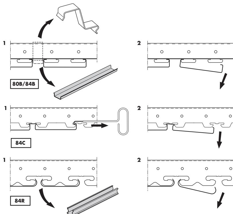
**GB** While demounting the panel make sure to support the part of the panel that has already been removed from the carriers.
